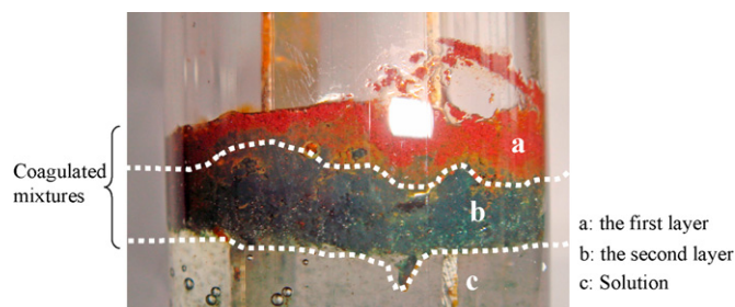
Fig. 3. Schematic diagram of the coagulated mixtures distribution in the electrochemical cell.
